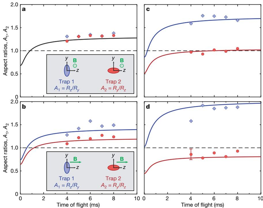
**Figure 4 | MDDI-dominated BEC expansion.** Aspect ratio of the condensate versus time of flight, for two traps with interchanged  $y$  and  $z$  frequencies (see text). The solid lines are theoretical predictions without adjustable parameters. The error bar (in **d**) gives the typical dispersion over several runs. **a**, Dipoles perpendicular to the observation plane (see inset sketching
