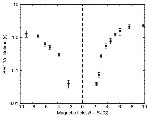
**Figure 2 | Inelastic losses close to the resonance.** The  $1/e$  lifetime of the condensate is plotted as a function of the magnetic field  $B$ . Error bars correspond to one standard deviation; the lifetime was determined by fitting the atom number remaining in the BEC after a variable holding time with an exponential decay law. The losses are small enough to allow for the observation of enhanced dipolar interactions (see Methods).
